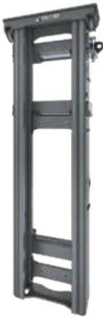
Duplex Standard NFL mast: 3000-7000 mm
